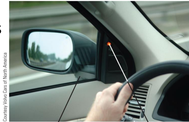
FIGURE 1-12 Embedded computers. This car's embedded computers control numerous features, such as notifying the driver when a car enters his or her blind spot.
