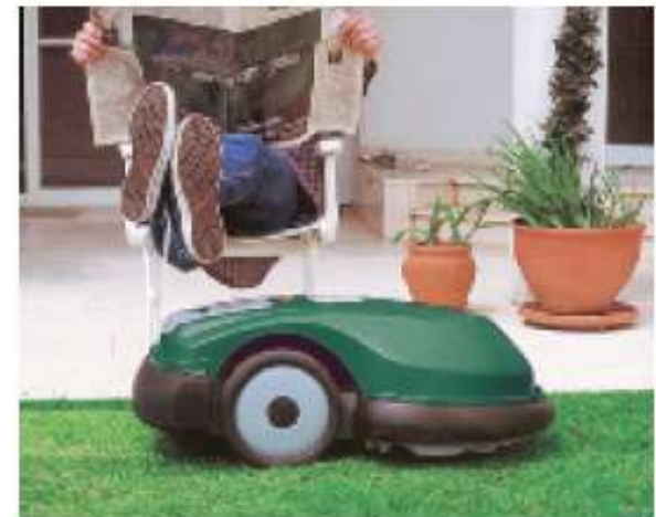
HELPER ROBOTS This robot is designed to automatically mow the lawn within a prescribed area.
