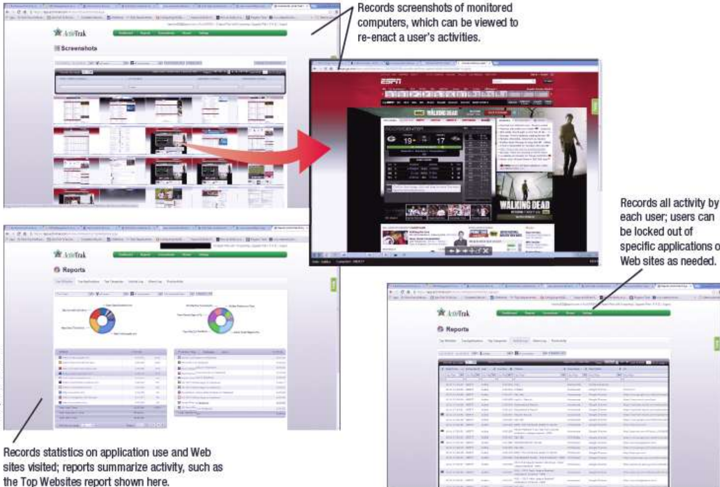
FIGURE 15-26 Computer monitoring software. Can be used to monitor employee computer activity, as shown here.
