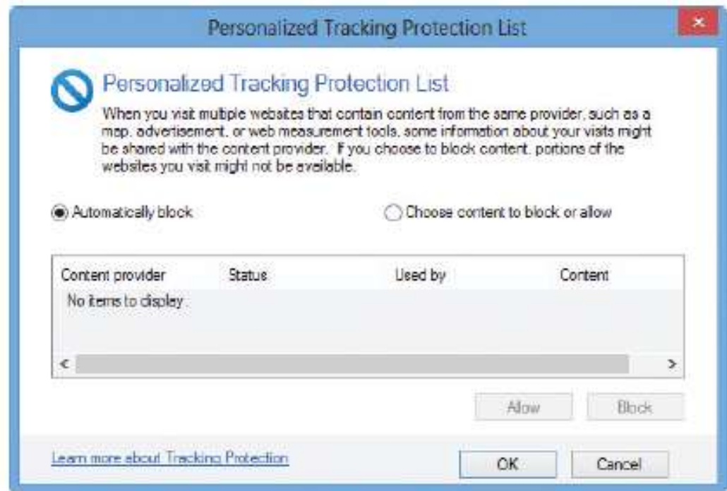
FIGURE 15-24 Enabling tracking protection in Internet Explorer.
