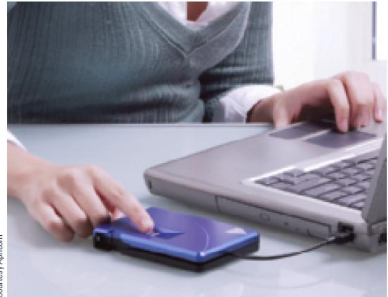
FIGURE 3-3 Encrypted hard drives. The data stored on this external hard drive is accessed via a fingerprint scanner.
