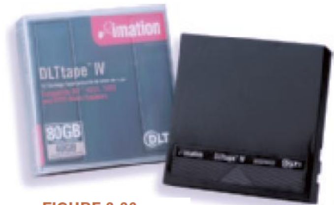
FIGURE 3-26 This magnetic tape cartridge holds 80 GB.
