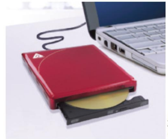
FIGURE 3-12 External optical drives. Can be connected as needed, typically via a USB port, such as to the netbook shown here.
