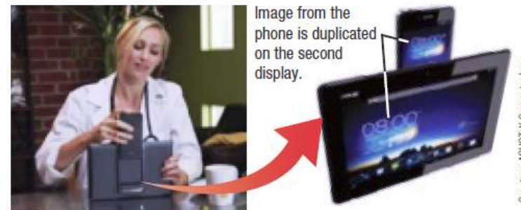
ADDITIONAL DISPLAYS FOR MOBILE DEVICES Typically duplicate the content displayed on the mobile device.
