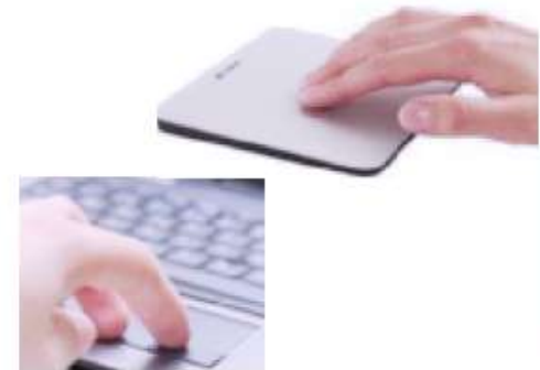
TOUCH PADS Commonly found on notebook and netbook computers (left); also available as stand-alone devices (right).
